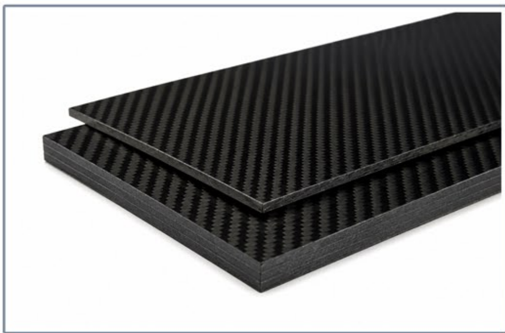
Composite specimen according to ASTM D5528
