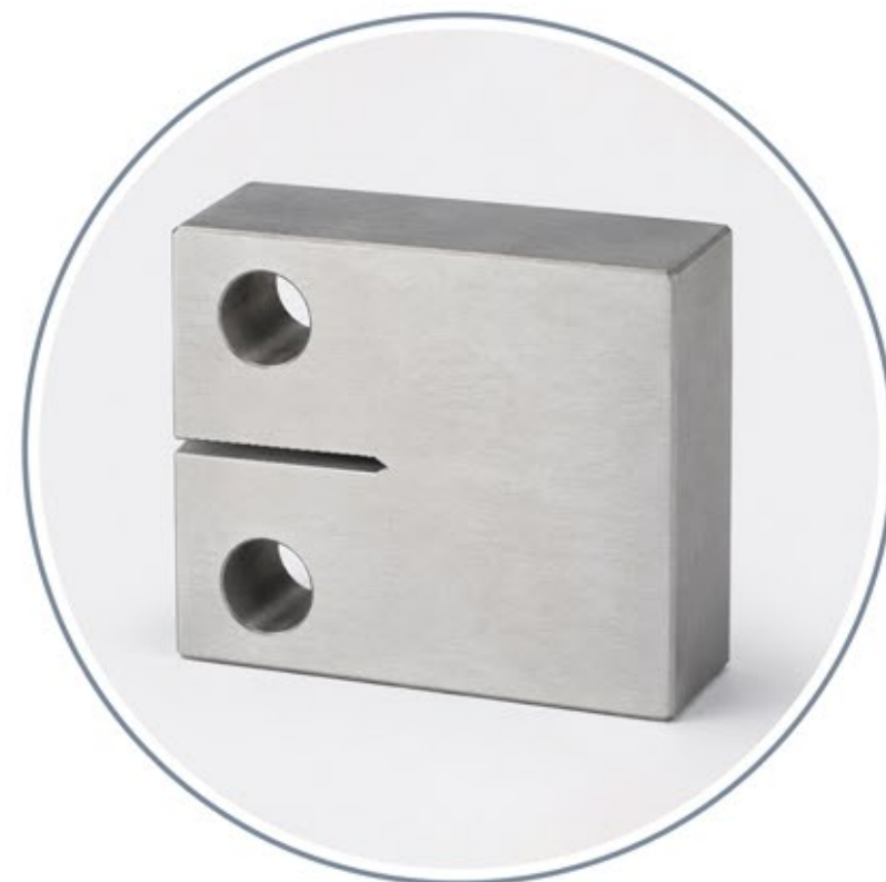
CT-specimen according to ASTM E399
