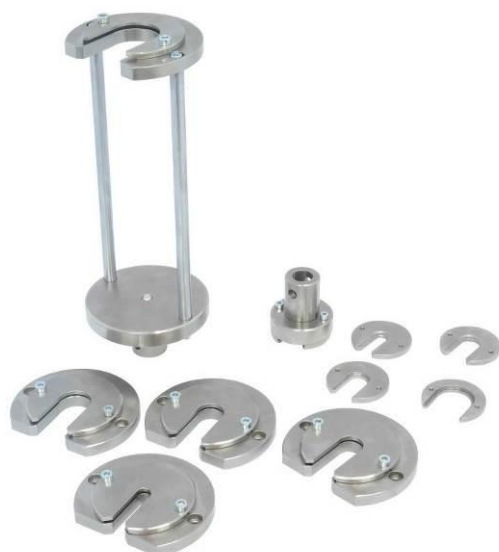
THS727-80 with inserts, upper part with adapter and inserts to accommodate syringes of different diameter
