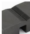
BV-jaws- for all kinds of round samples - Tooth pitch 1.2 mm - Hardened steel 58 HRC, nickel plated
