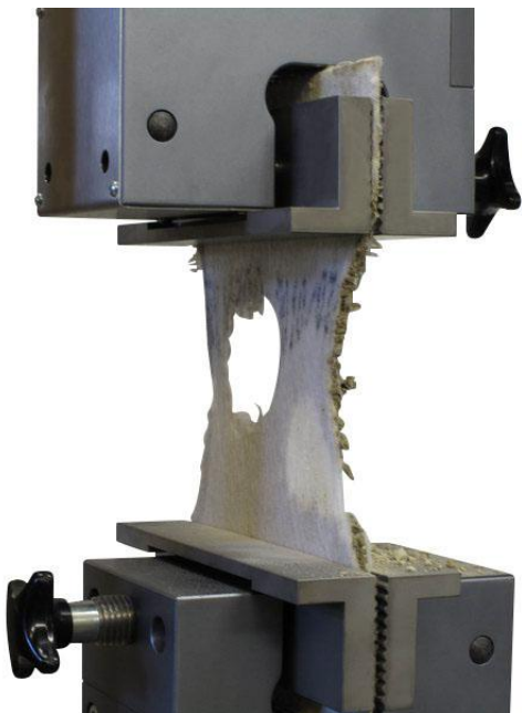
TH126+BW200: Wave jaws 60 x 200 mm, test with carpet sample
