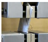
Felt tensile test under angle http://www.youtube.com/watch?v=GZg1XtvVmwg
