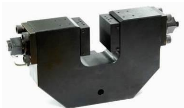
TH135-60-d symmetric design, double-action cylinder
