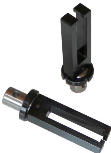
TH16-S18-Am32 according to ASTM D143 to test small clear specimens of timber
