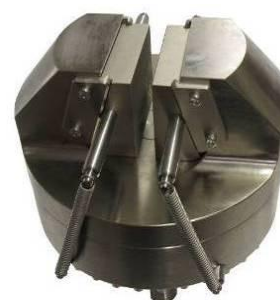
TH175-100-D260-S46 Extra wide jaw opening 46 mm
