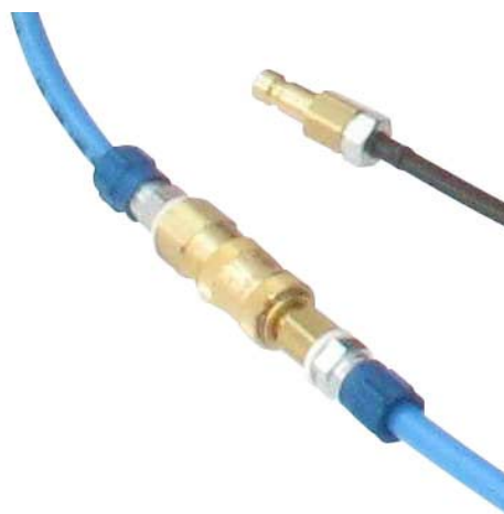
TH205-9 Mini plug (total length plugged together: 30 mm, external Ø 10 mm, M5 thread)
