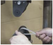
How to insert and fix a ribbon in TH222
