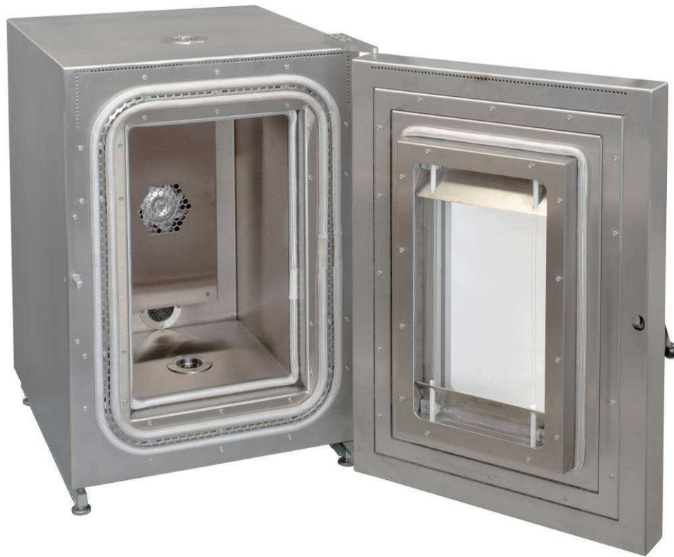
TK389 T500°C special chamber for useage up to 500°C
