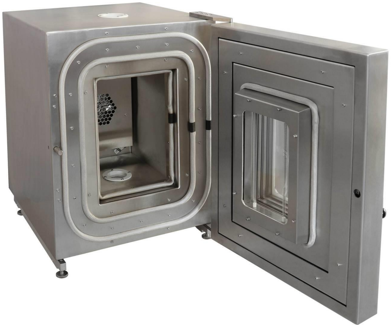
TK332 -180°C innen 220x230x310mm 120mm Wallthickness
