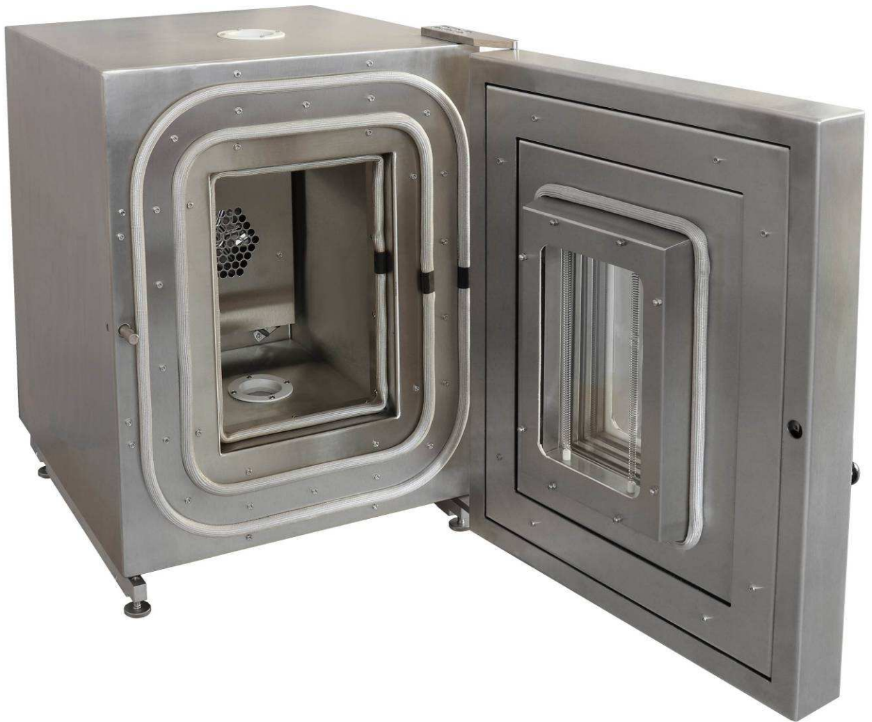
TK332 -180°C innen 220x230x310mm 120mm Wallthickness
