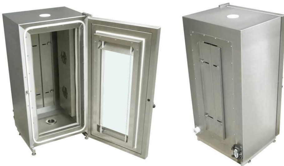
TK190-LHB long hole on back side for long travel extensometer
