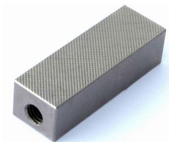
THS13m-BP0.5 Special jaws. Fine pyramids, cross cut 0.5x45° Nickel coated T range -70°C to +180°C
