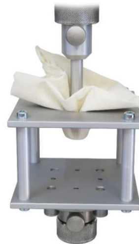
THS174-35H60-FD15 to determine stiffness of fabric according to ASTM D4032
