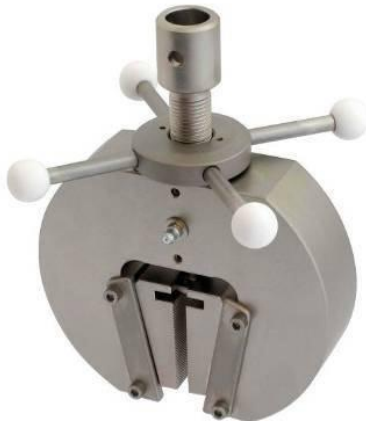
THS527-20-T280 20 kN, temperature range -70...280°C
