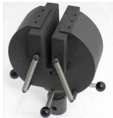
THS527-50+BP125 with special wide jaws 125x100 mm
