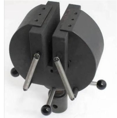
THS527-50+BP125 with special wide jaws 125x100 mm
