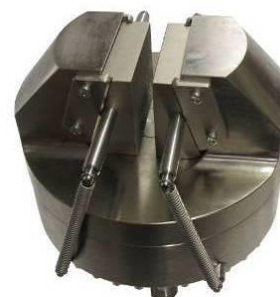
TH175-100-D260-S46 Extra wide jaw opening 46 mm
