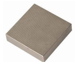
THS22-BP0.8x45 Pyramid jaws 50x50 mm with 0.8x45 pyramids
