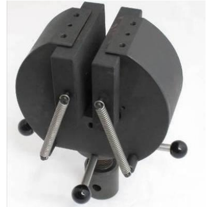
THS527-50+BP125 with special wide jaws 125x100 mm
