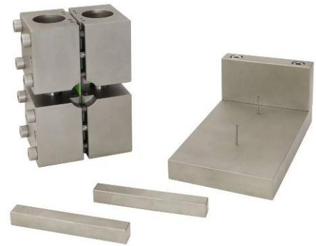
THS705-2G with alignment bars and sample positioning tool
