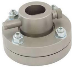
THS223g-96-St. 96 mm Ø. Steel, nickel-plated Spherically-seated compression platen, self-aligning and fixable
